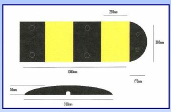
This **Rubber Speed Hump** offers a low-cost solution in installations where traffic flows are not excessive. This is a modular system that can be supplied to any required length, with end caps supplied to suit the required layout. These speed humps offer particularly smooth and silent operation, and are recommended for use around residential apartments, hospitals, schools, shopping centres and commercial/retail buildings.
