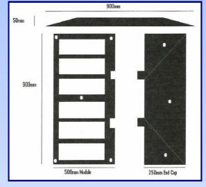
This is a 900mm wide **Rubber Speed Hump** specifically for the purpose of reducing vehicle speed rather than bringing vehicles to a complete stop. This has the effect of reducing fleet fuel consumption over a standard speed hump, as well as reducing noise from vehicle acceleration.
