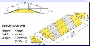
**Heavy-Duty Steel Speed Humps** are the preferred choice for industrial premises and warehouses, where there are high traffic flows and commercial vehicles. These humps are suitable for use with trucks and other heavy-vehicles (including 'B—doubles'). This speed hump system is modular in design, and comes fully zinc plated and painted for many years of trouble free service.
