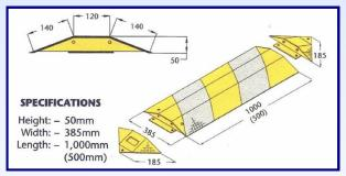
**Steel Speed Humps** are designed for higher traffic flows, and our designs minimize noise and 'rattle'. These units are suitable for passenger cars and light commercial vehicles, but are not recommended for use with heavy-vehicles.
